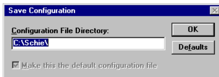
This dialog box displays the path where the Server is going to save the current configuration file. The path may be changed if necessary. Also, the path can optionally be recorded in the **WIN.INI** file by selecting the **"Make this the default configuration file"**
